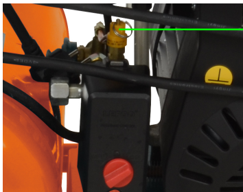
Figure 5: Safety valve
