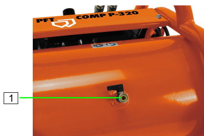
Figure 11: Open the bleed valve
