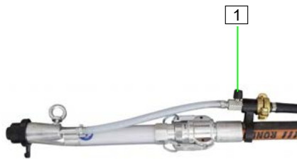
Figure 40: Closing the air tap
