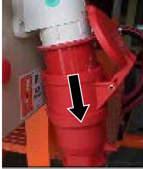
Figure 60: Remove connection cable
