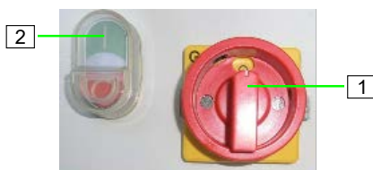
Figure 46: Switching on the machine after a power failure
