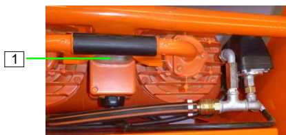
Figure 42: Switching off the air compressor
