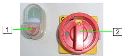
Figure 43: Switching off the machine
