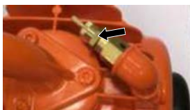
Figure 63: Safety valve
