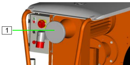
Figure 33: Change motor speed
