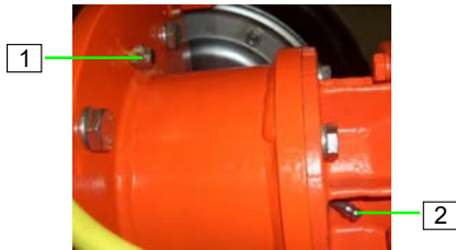
Figure 61: Sealing unit
