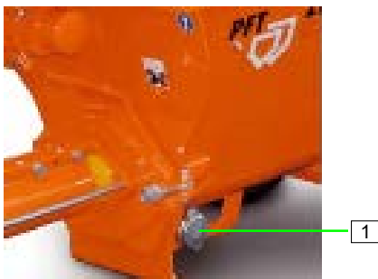
Figure 24: Opening the cleaning nozzles
