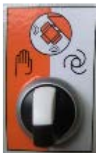
Figure 15: Selector switch - Vibrating unit
