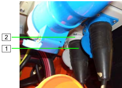
Figure 66: Connect booster pump
