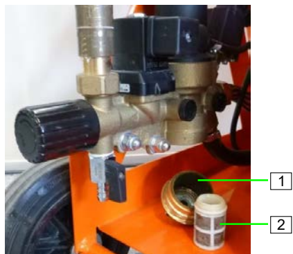
Figure 128: Strainer screen in pressure reducer
