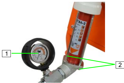
Figure 121: Checking the grout pressure
