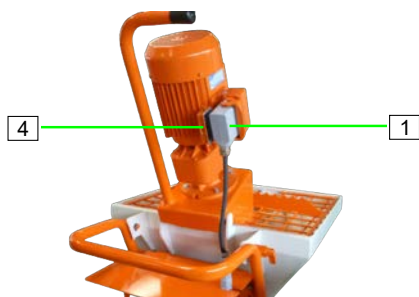
Figure 108: Remove the motor connection cable
