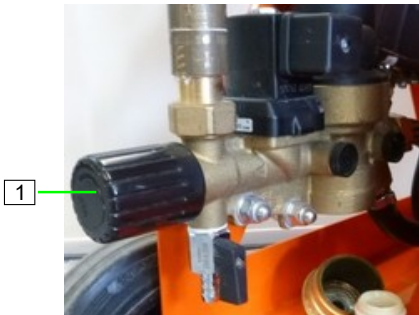
Figure 129: Pressure reducing valve
