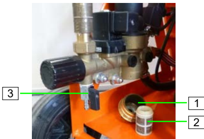
Figure 44: Checking the strainer screen
