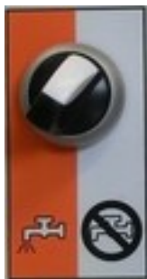
Figure 29: Water selector switch
