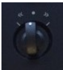
Figure 26: Pump motor selector switch
