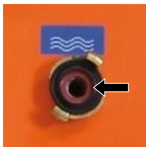
Figure 127: Strainer screen in the water inlet
