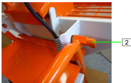
Figure 7: Opening the rotary bolt
