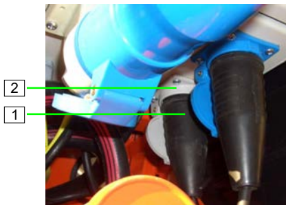
Figure 64: Connecting the vibrating unit
