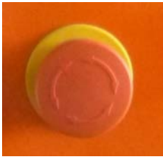
Figure 23: EMERGENCY STOP / EMERGENCY OFF button
