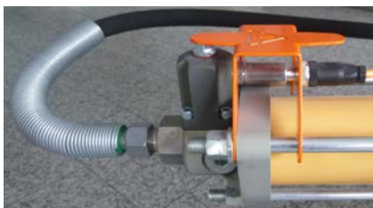
Figure 24: Pressure sensor
