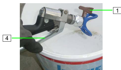
Figure 90: Clean the reversing nozzle
