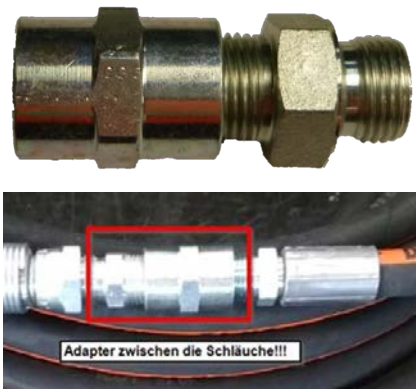
Figure 35: Adapter between hoses
