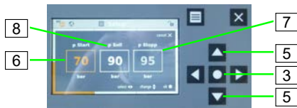
Figure 44: Setting the switch-on and switch-off pressure
