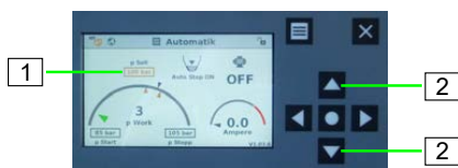
Figure 44: Setting the switch-on and switch-off pressure
