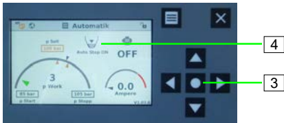
Figure 46: Activate idle protection
