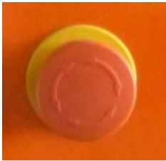
Abb. 23: NOT-HALT/NOT-AUS-Taster
