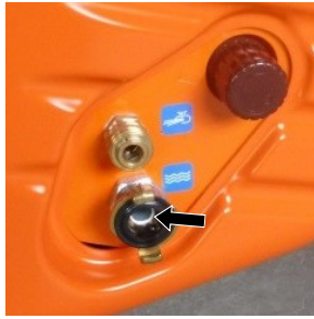
Figure 130: Strainer screen in the water inlet
