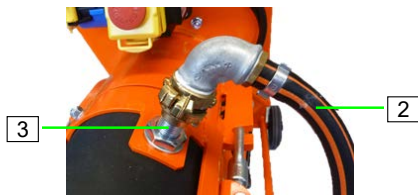
Figure 36: Disconnect water supply
