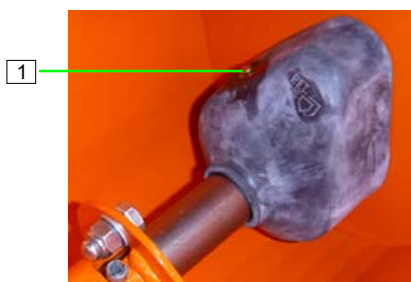
Figure 48: Lubricate the bearings
