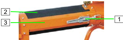
Figure 41: Cleaning the mixing tube
