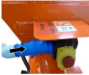
Figure 17: Connect power supply
