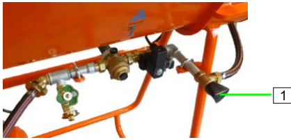
Figure 25: Setting the water quantity
