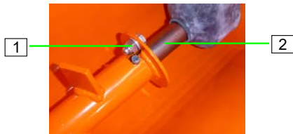
Figure 44: Cleaning the dosing shaft
