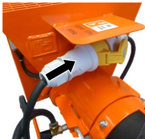
Figure 18: Connect power supply
