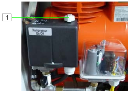
Figure 74: Switching off the air compressor
