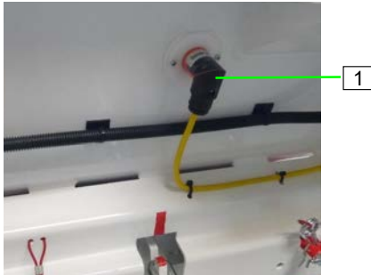
Figure 33: Level sensor in the mixer
