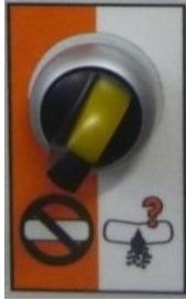
Figure 17: Level sensor selector switch
