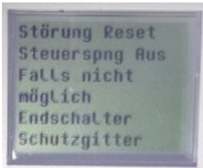
Figure 100: Fault limit switch protective grille
