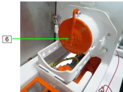
Figure 91: Closing the mixing tube cover
