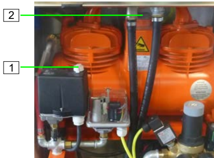
Figure 60: Switching on the air compressor
