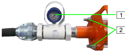
Figure 78: Check and relieve the mortar pressure
