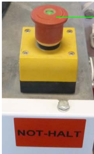
Figure 29: EMERGENCY STOP / EMERGENCY OFF button
