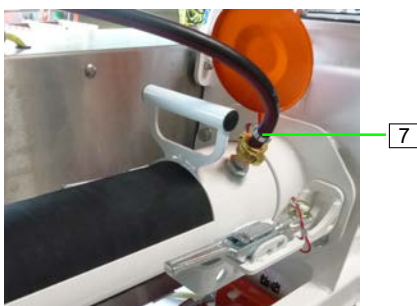
Figure 46: Connecting the water hose
