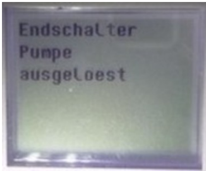
Figure 99: Fault limit switch pump unit
