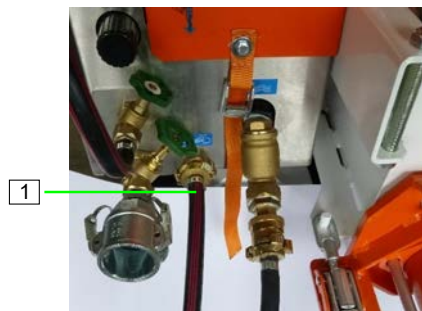
Figure 58: Connecting the air hose
