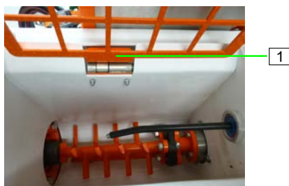
Figure 32: Hinge safety switch
