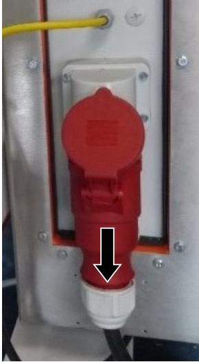
Figure 105: Remove connection cable
