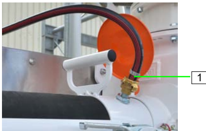
Figure 81: Remove the water hose
