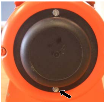
Figure 107: Removing the filter cover
