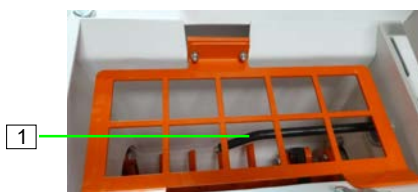
Figure 62: Wet sensor
