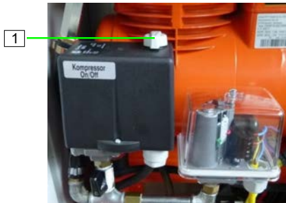
Figure 67: Switching off the air compressor
