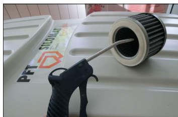
Fig. 53: Cleaning the filter cartridges
