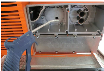
Fig. 54: Cleaning filter housing
