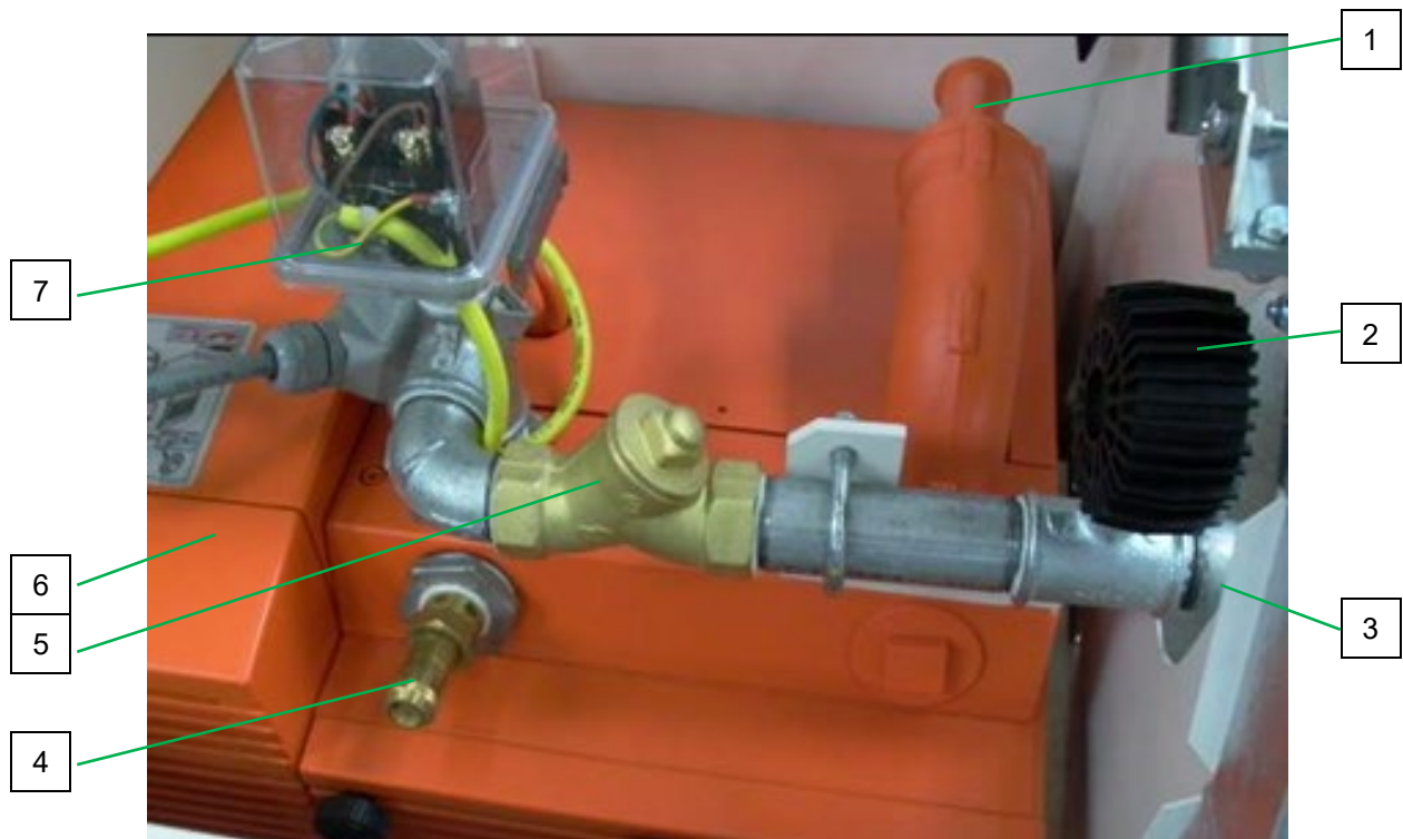
Fig. 6: Overview of rotary compressor / pressure control
