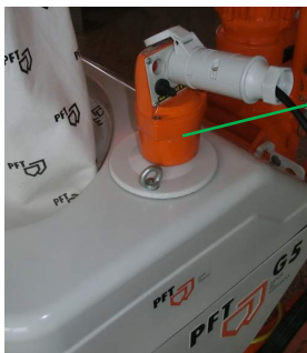
Fig. 37: Pulling off control plug
