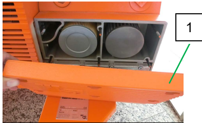
Fig. 51: Loosen filter cover
