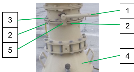
Fig. 39: Removing conveying vessel
