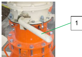
Fig. 37: Close the silo discharge flap valve
