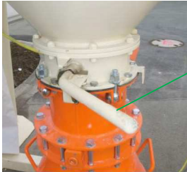
Fig. 30: Close the silo discharge flap valve
