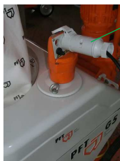
Fig. 34: Remove control plug
