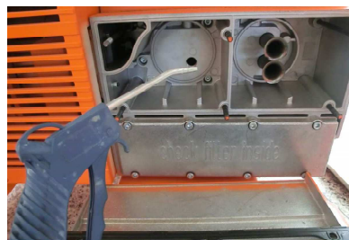
Fig. 48: Clean the filter housing
