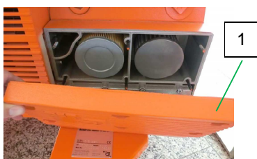
Fig. 45: Remove the filter cover
