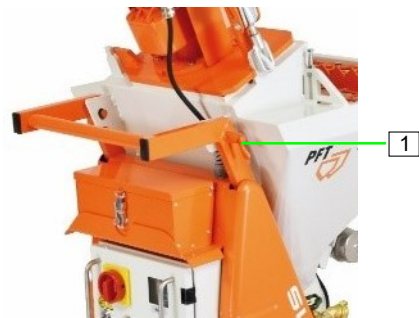
Figure 7: Opening the rotary bolt
