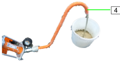
Figure 58: Checking the consistency
