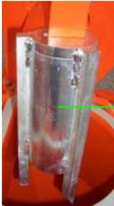
Figure 83: Inserting the mixing tube cleaner
