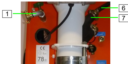
Figure 42: Water sampling valve
