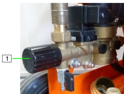
Figure 99: Pressure reducing valve
