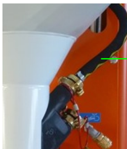
Figure 81: Connecting the water hose
