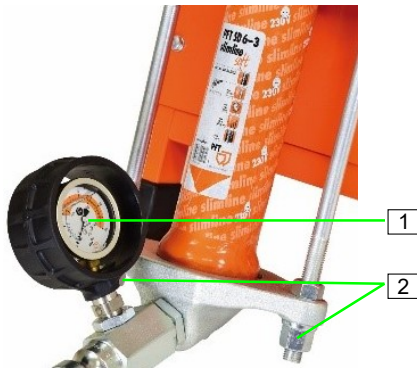
Figure 71: Check and relieve the mortar pressure
