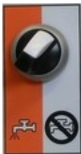
Figure 22: Water selector switch
