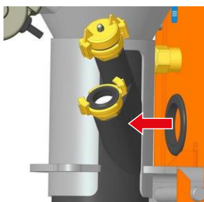
Figure 89: Seating of the rubber mixing zone
