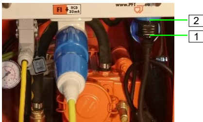
Figure 50: Switching on the air compressor
