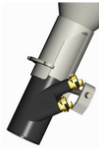
Figure 88: Cleaning the rubber mixing zone
