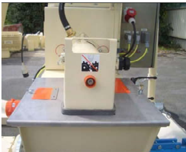
Fig. 70: Installing mixing tube
