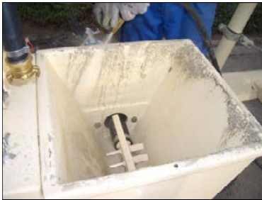
Fig. 68: Cleaning the pump container
