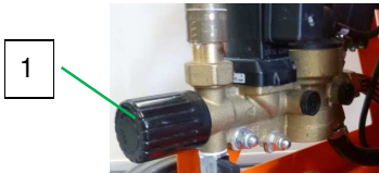
Fig. 100: Pressure reducing valve
