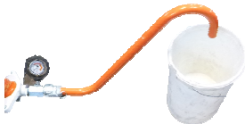
Fig. 54: Consistency checking tube
