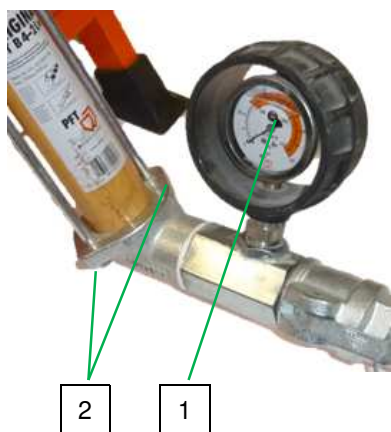
Fig. 72: Check mortar pressure
