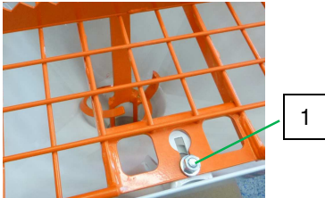
Fig. 27: Tighten the nuts
