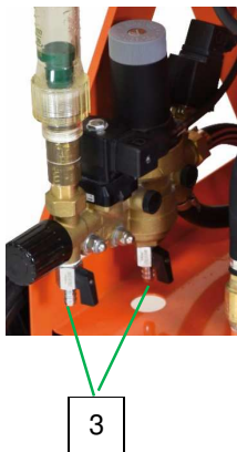
Fig. 95: Opening the drain tap
