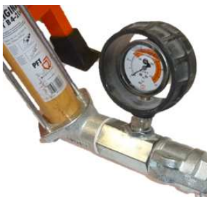
Fig. 51: Mortar pressure gauge
