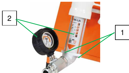
Fig. 93: Remove pump unit
