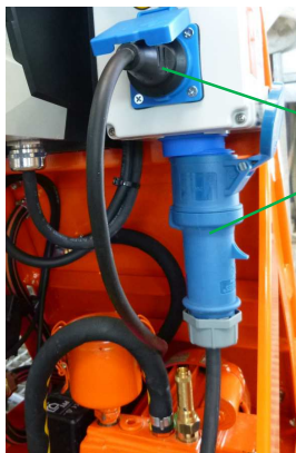
Fig. 96: Remove connection cable
