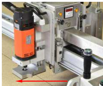
Fig. 11.02 milling cutter unit left
