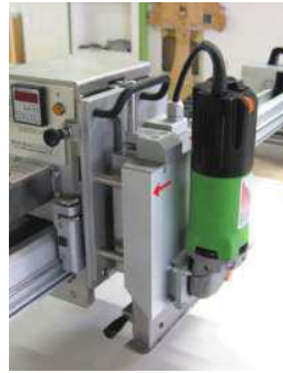
Fig. 15.03 Cross cutting unit
