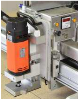
Fig. 15.01 Milling cutter unit
