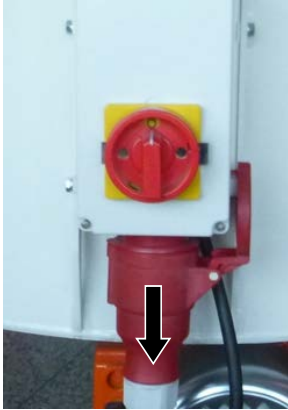
Figure 31: Remove connection cable
