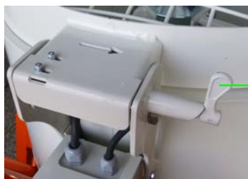
Figure 32: Grease the rotary bolt
