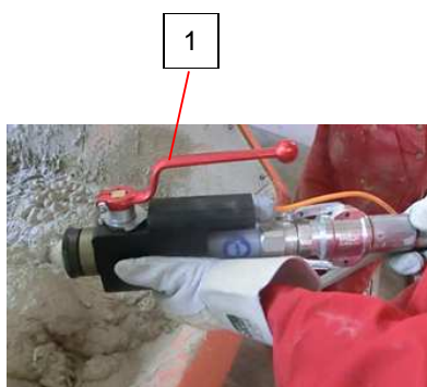
Fig. 9: Open the hand lever
