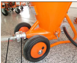
Fig. 4: Connect material hose
