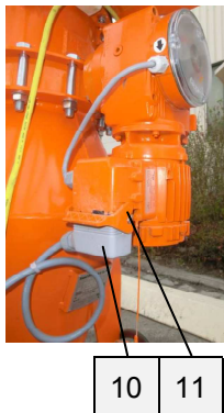
Fig. 7: Connection actuator
