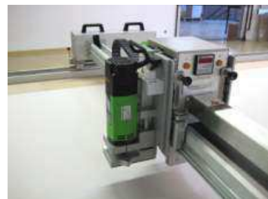
Fig. 11.02 Milling unit, left
