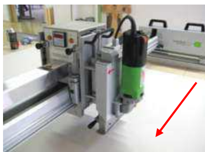
Fig. 11.05 Sawing unit, transverse, right
