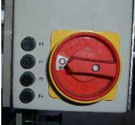
Main switch 0-1 with undervoltage trigger.
