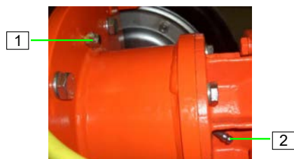
Figure 60: Sealing unit
