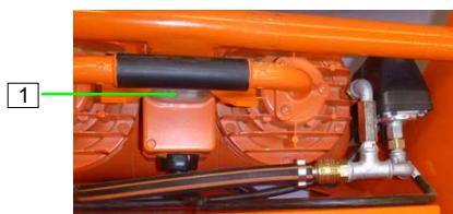
Figure 40: Switching off the air compressor
