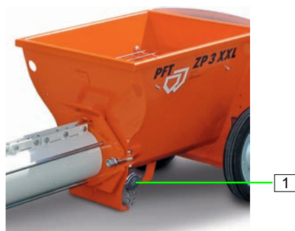
Figure 51: Opening the cleaning nozzles
