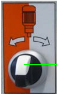
Figure 35: Switching on
