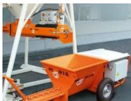
Figure 30: Loading the ZP 3 with material
