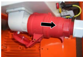
Figure 59: Remove connection cable
