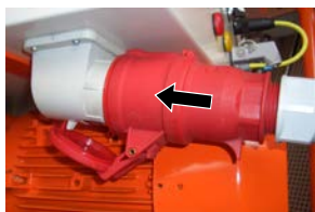
Figure 21: Connecting the power supply
