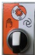
Figure 15: Selector switch - Vibrating unit
