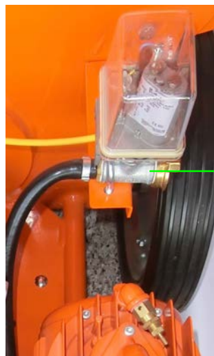
Figure 28: Connecting the air hose
