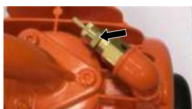
Figure 62: Safety valve
