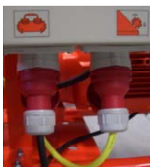
Fig. 20: Connect vibrator and air compressor together
