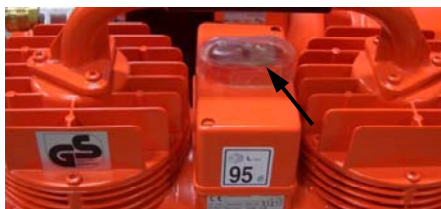
Fig. 34 Open the spray device air cock
