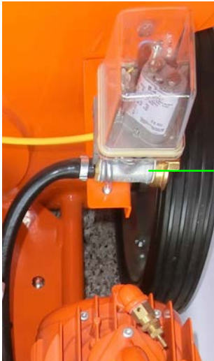
Figure 32: Connecting the air hose
