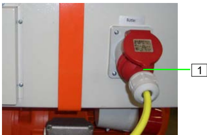
Figure 26: Power connections
