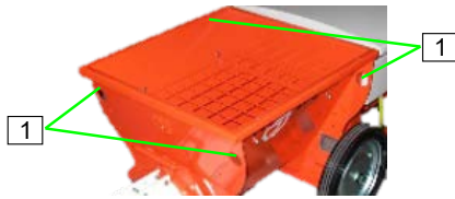
Figure 5: Attachment points for crane transport
