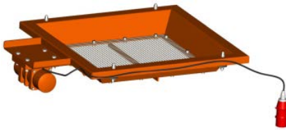
Figure 15: Vibrating screen
