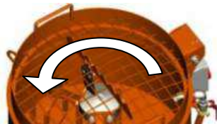
Fig. 25: Checking the direction of rotation
