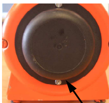
Fig. 82: Filter cover opening
