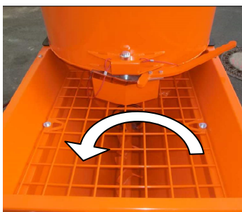
Fig. 31: Checking the direction of rotation
