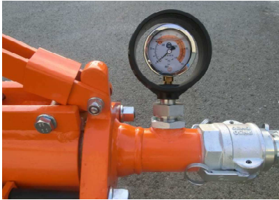
Fig. 24: Mortar pressure gauge
