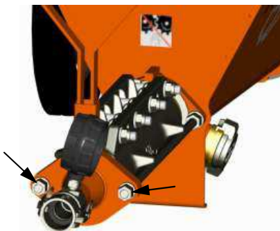
Fig. 71: Releasing the nuts
