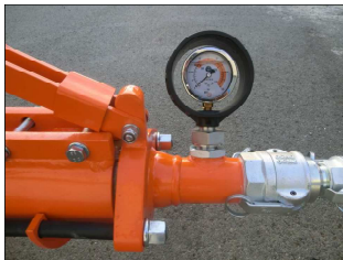
Fig. 19: Mortar pressure gauge
