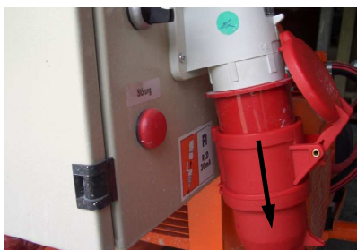
Fig. 76: Removing the connection cable
