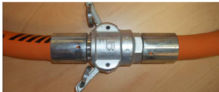
Fig. 69: Detaching connections
