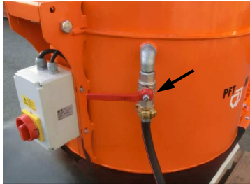
Fig. 28: Water connection
