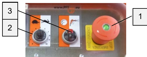
Fig. 41: Selector switch pump motor
