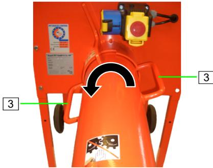
Figure 39: Removing the mixing tube
