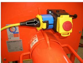
Figure 22: Connect power supply.
