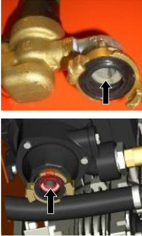
Figure 46: Strainer screen in the water inlet
