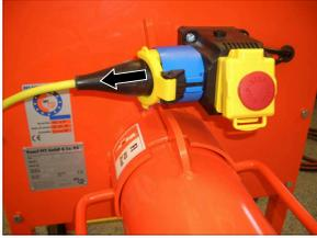
Figure 45: Remove connection cable
