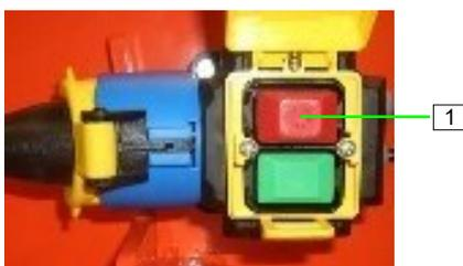
1. Switch off the machine by pressing the red "OFF" pushbutton (1).
