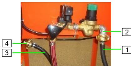
Figure 37: Disconnect water supply
