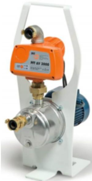
Water pump as standalone suction pump AV 1000 with integrated pressure cut-off and flow monitor, 230 V, 1 Ph, 50 Hz, 0.6 kW
