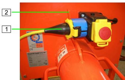
1. Disconnect the power supply, remove the connection cable (1).
