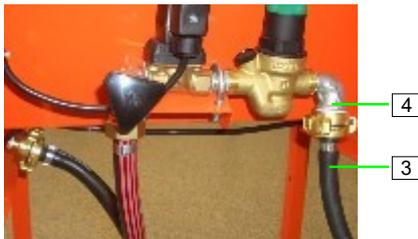
Figure 25: Connecting water supply
