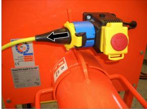
Figure 35: Disconnecting the power supply
