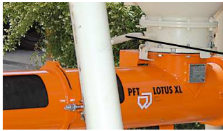
Fig. 39: Closing the silo outlet flap
