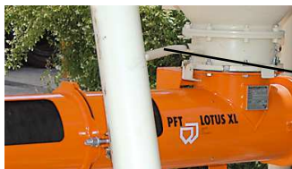
Fig. 34: Opening the silo outlet flap
