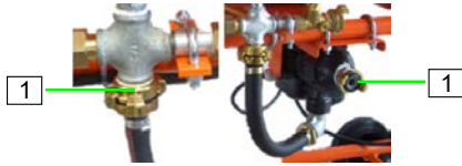
Figure 52: Strainer screen in the water inlet
