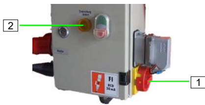
Figure 22: Checking the direction of rotation
