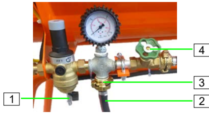
Figure 25: Water supply connection without a booster pump
