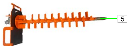
Figure 45: Greasing the bearing journal
