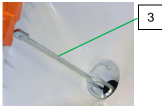
Fig. 107: Removing the mixing shaft
