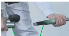
Fig. 101: Removing the pump unit
