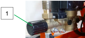
Fig. 115: Pressure reducing valve
