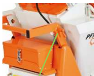
Fig. 32: Opening the rotary bolt
