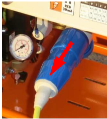
Fig. 111: Removing the connection cable
