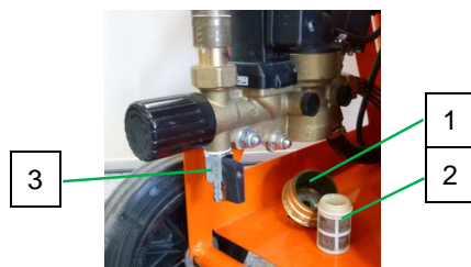
Fig. 39: Dirt trap screen
