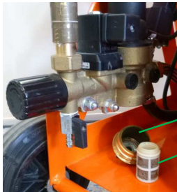
Fig. 114: Dirt trap screen
