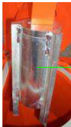
Figure 78: Inserting the mixing tube cleaner
