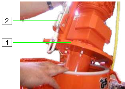
Figure 5: Closing the motor tilt flange
