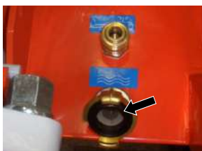
Figure 96: Strainer screen in the water inlet
