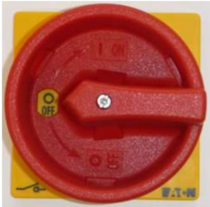
Figure 64: Turn main switch to the "OFF" position
