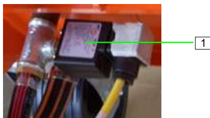
Figure 99: Pressure switch air
