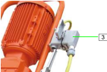
Figure 32: Connecting the motor connecting cable
