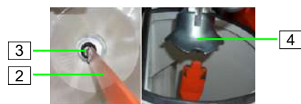
Figure 79: Cleaner shaft seat
