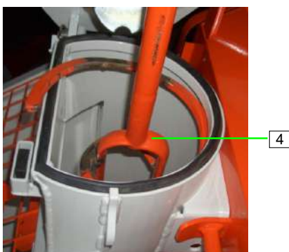
Figure 77: Removing the mixing shaft
