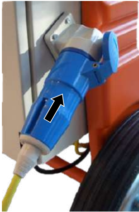
Figure 30: Connecting the power supply
