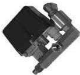
Figure 100: Air compressor pressure cut-off
