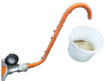
Figure 53: Consistency inspection tube
