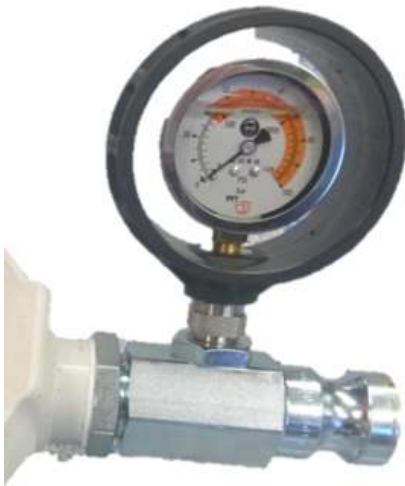
Figure 17: Mortar pressure gauge
