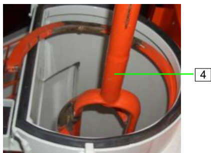
Figure 68: Removing the mixing shaft
