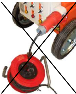
Figure 29: Image showing example of impermissible connection variant
