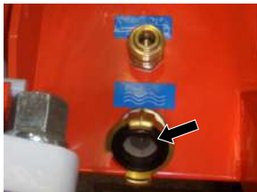
Figure 94: Strainer screen in the water inlet
