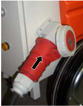
Figure 32: Connecting the power supply
