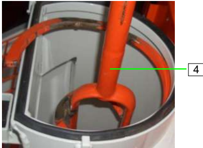
Figure 70: Removing the mixing shaft
