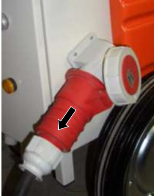
Figure 92: Remove connection cable
