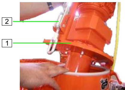
Figure 82: Closing the motor tilt flange
