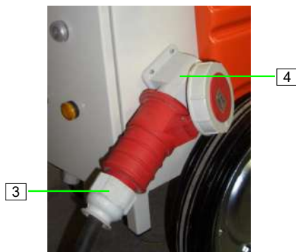
Figure 30: Connecting the power supply
