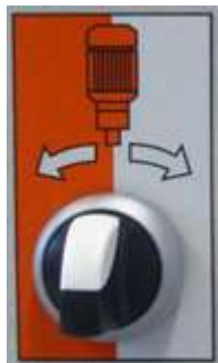
Figure 19: Pump motor selector switch
