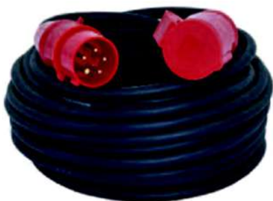
Extension cable 5 x 4 mm², RED 5-32 A – 50 m (400 V, 3 Ph)
