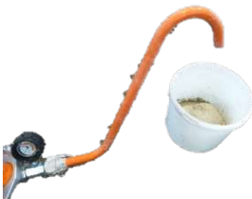
Figure 55: Consistency inspection tube
