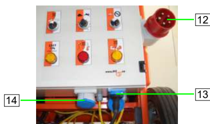
Figure 14: Assembly unit control box
