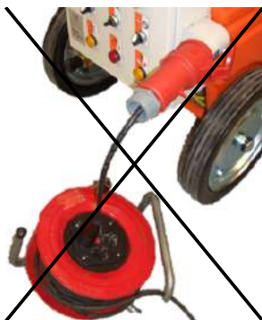
Figure 31: Image showing example of impermissible connection variant
