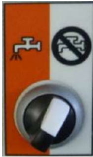
Figure 20: Water selector switch
