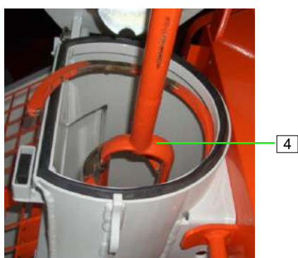
Figure 79: Removing the mixing shaft
