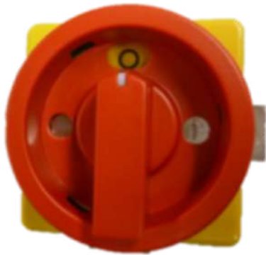
Figure 66: Turn the main reversing switch to the "0" position
