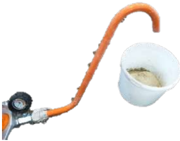
Figure 45: Consistency inspection tube
