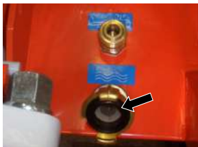
Figure 85: Strainer screen in the water inlet
