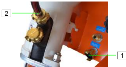
Figure 29: Connecting the water
