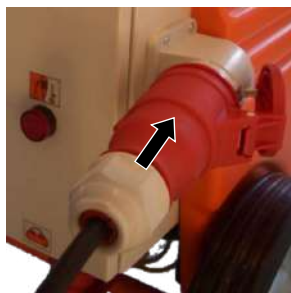
Figure 25: Connecting the power supply
