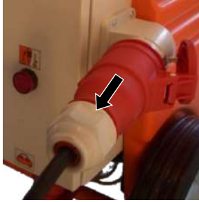
Figure 82: Remove connection cable
