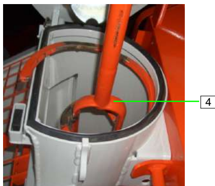
Figure 69: Removing the mixing shaft
