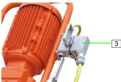
Figure 27: Connecting the motor connecting cable
