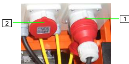
Figure 26: Power connections
