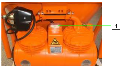
Figure 45: Switching on the air compressor
