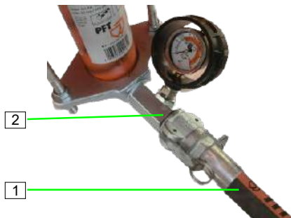
Figure 41: Connecting the mortar hose
