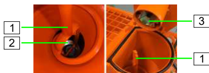
Figure 79: Inserting the mixing shaft
