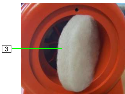
Figure 87: Filter of the air compressor
