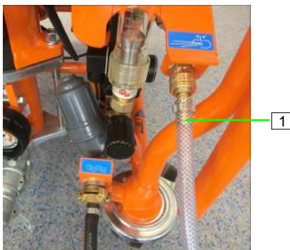
Figure 43: Connecting the air hose
