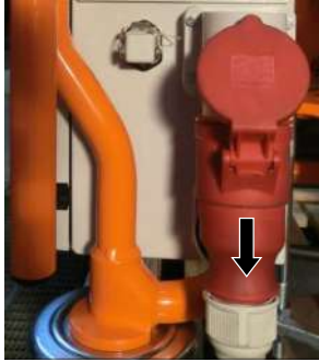
Figure 85: Remove connection cable
