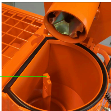
Figure 72: Opening the motor tilt flange
