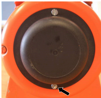
Figure 85: Filter cover opening
