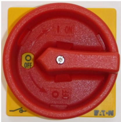
Figure 59: Turn main switch to the "OFF" position
