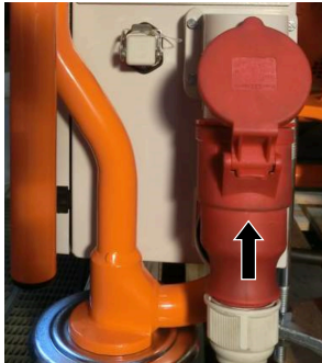
Figure 29: Connect power supply.
