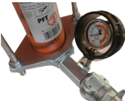
Figure 26: Mortar pressure gauge
