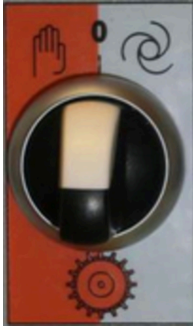
Figure 18: Selector switch star wheel
