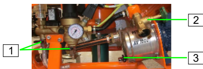
Figure 31: Closing the drainage cocks
