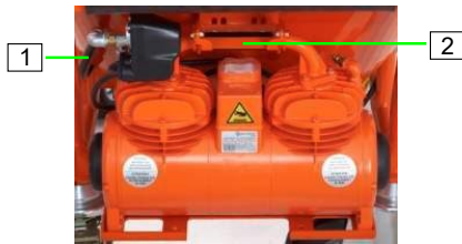
Figure 83: Remove air compressor
