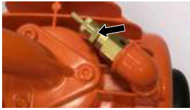
Figure 90: Safety valve
