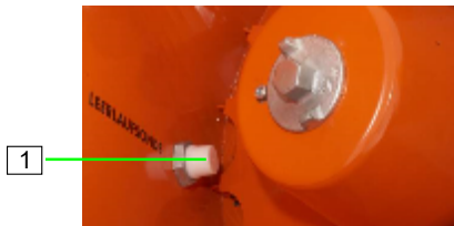
Figure 24: Level sensor in the material hopper
