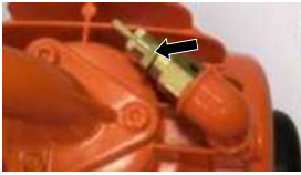
Figure 94: Safety valve
