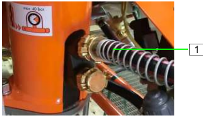
Figure 75: Connecting the water hose
