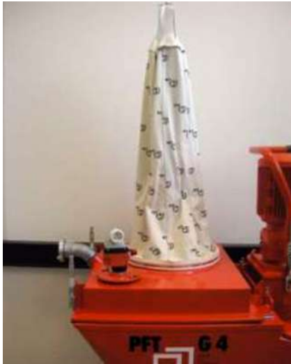
Figure 49: Injection hood
