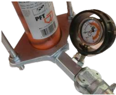
Figure 17: Mortar pressure gauge
