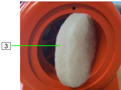
Figure 88: Filter of the air compressor
