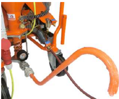
Figure 53: Consistency inspection tube
