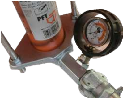
Figure 27: Mortar pressure gauge
