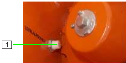
Figure 27: Level sensor in the material hopper
