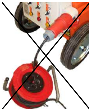
Figure 34: Image showing example of impermissible connection variant
