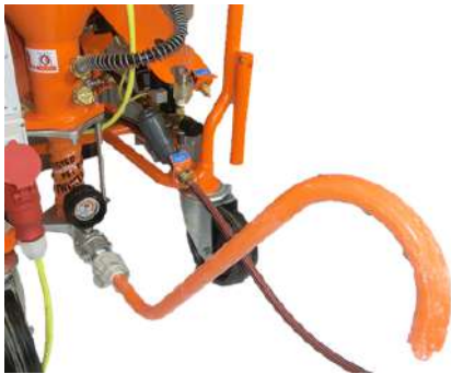
Figure 57: Consistency inspection tube
