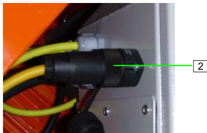
Figure 28: Deactivate level sensor
