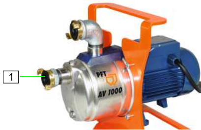
Figure 54: Filling the pump
