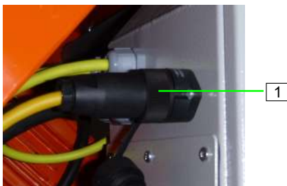
Figure 75: Deactivate level sensor
