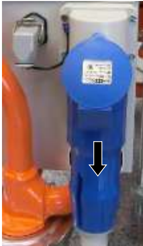
Figure 91: Remove connection cable
