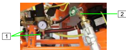
Figure 37: Closing the drainage cocks
