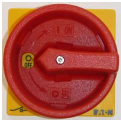
Figure 68: Turn main switch to the "OFF" position
