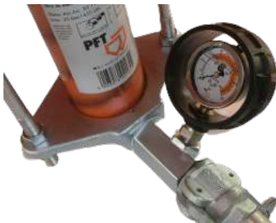
Figure 17: Mortar pressure gauge
