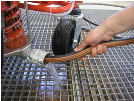
Fig. 47: Rinsing out deposits
