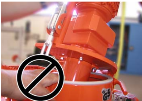
Fig. 43: Close the motor tilt flange
