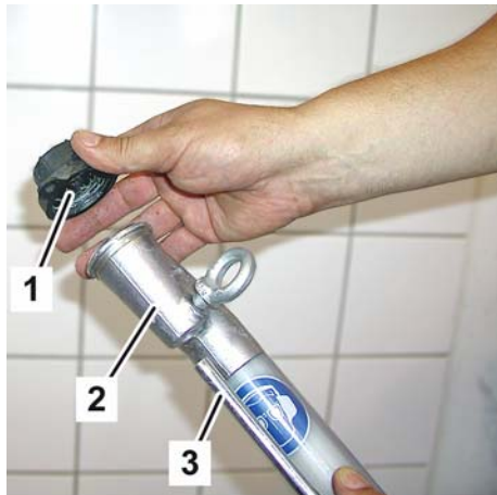
Fig. 50: Air nozzle pipe and plaster nozzle
