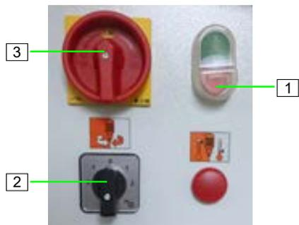
1. Switch off the machine by pressing the red pushbutton (1) control voltage 'OFF'.
