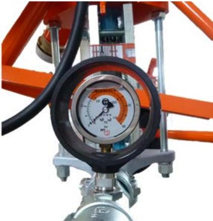
Figure 17: Mortar pressure gauge
