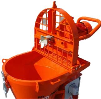
Figure 5: Closing the motor tilt flange
