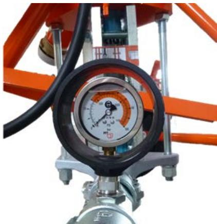
Figure 14: Mortar pressure gauge
