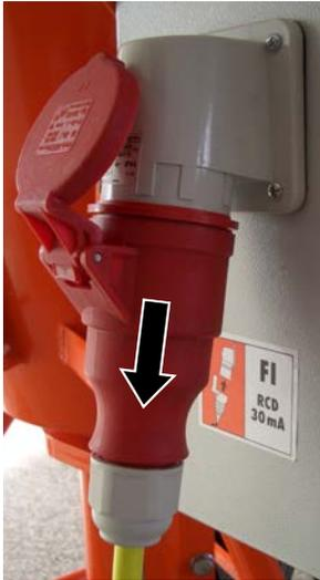
Figure 47: Remove connection cable
