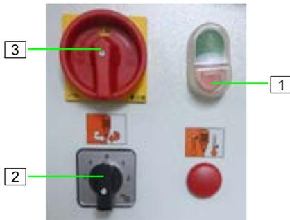
1. Switch off the machine by pressing the red pushbutton (1) control voltage 'OFF'.
