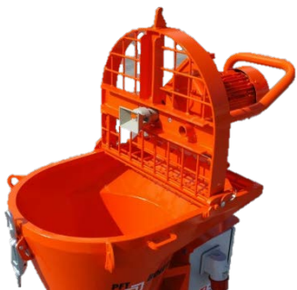
Figure 4: Closing the motor tilt flange
