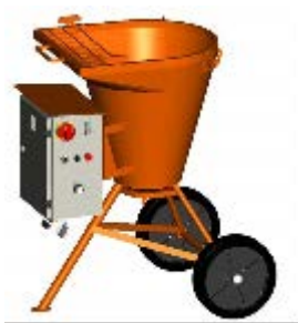
Figure 11: Material hopper assembly
