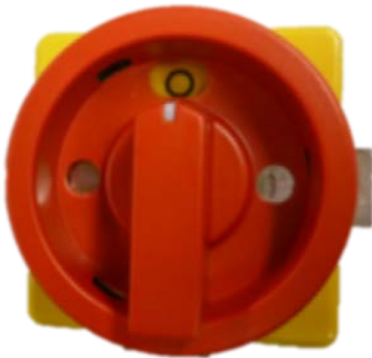
Figure 28: Turn the main reversing switch to the "0" position
