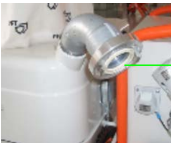
Figure 19: Connecting the conveying hose
