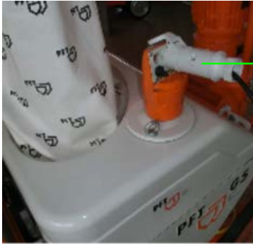
Figure 30: Remove control plug
