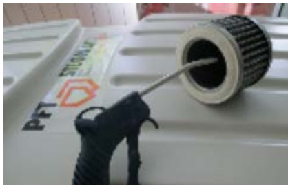
Figure 61: Clean the filter cartridges
