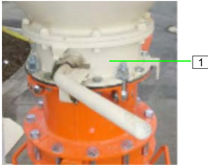
Figure 22: Opening the silo discharge flap valve
