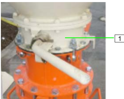
Figure 32: Closing the silo discharge flap valve
