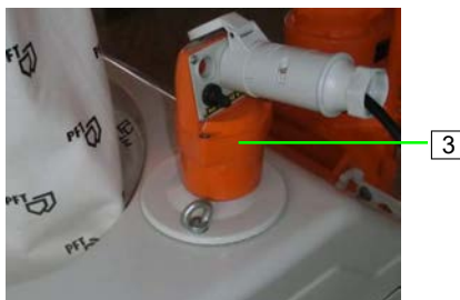
Figure 16: Connecting the control cable
