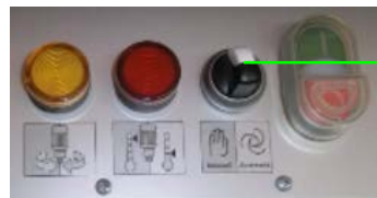
Figure 42: Blow out the conveying hoses
