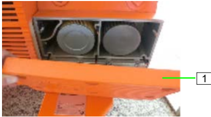
Figure 59: Remove the filter cover
