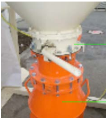
Figure 18: Connecting the carrier
