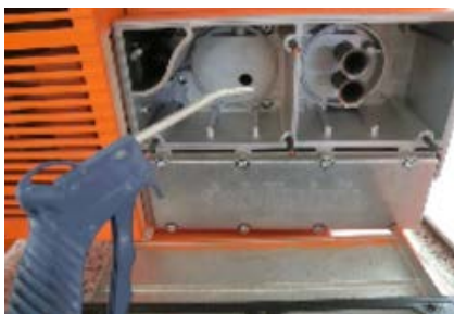
Figure 62: Clean the filter housing
