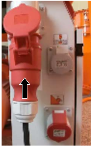
Figure 14: Connect power supply.
