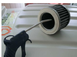
Fig. 38: Clean the filter cartridges
