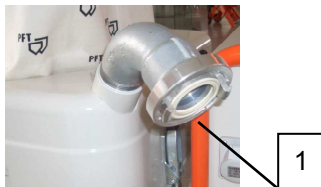
Fig. 9: Connecting the conveying hose
