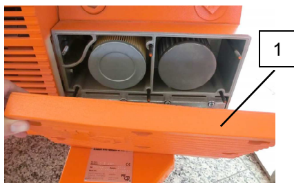
Fig. 36: Remove the filter cover
