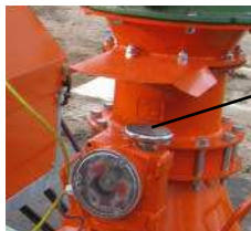
Fig. 19: Opening the shut-off flap valve
