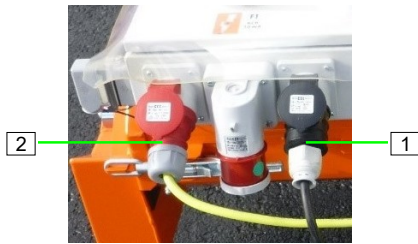
Abb. 18: Stromanschlüsse
